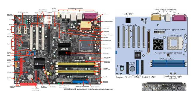
Picture of a motherboard/logicboard
