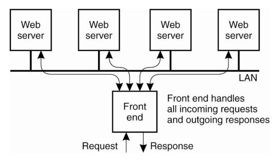
• The principle of using a server cluster in combination with a front end to implement a Web service.
