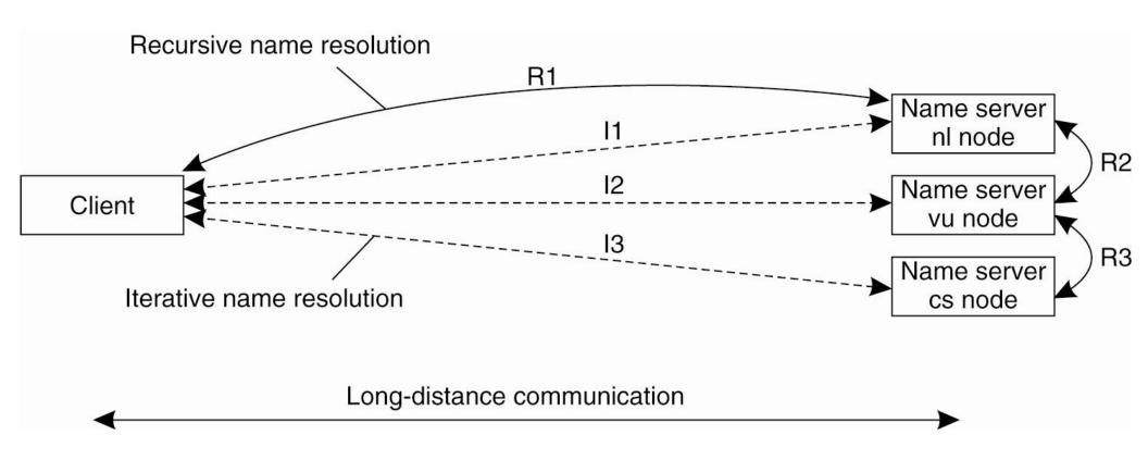
• Comparison between recursive and iterative name resolution with respect to communication costs.
