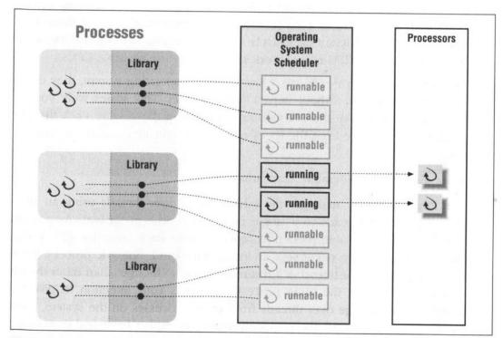
Figure 6-2: Kernel thread-based implementations
