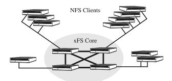
Figure 7. An xFS core acting as a scalable file server for unmodified NFS clients.
