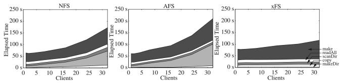
Figure 11. Average time to complete the Andrew benchmark for NFS, AFS, and xFS as the number of clients simultaneously executing the benchmark varies. The total height of the shaded areas represents the total time to complete the benchmark; each shaded area represents the time for one of the five phases of the benchmark: makeDir, copy, scanDir, readAll, and make. For all of the systems, the caches were flushed before running the benchmark.
