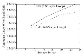
Figure 12. Large write throughput as a function of the number of storage servers in the system. The x axis indicates the total number of storage servers in the system and the y axis indicates the aggregate bandwidth when 32 clients each write a 10 MB file to disk. The 8 SS's line indicates performance for stripe groups of eight storage servers (the default), and the 4 SS's shows performance for groups of four storage servers.
