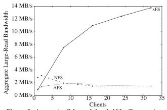
**Figure 9.** Aggregate disk read bandwidth. The x axis indicates the number of clients simultaneously reading private 10 MB files and the y axis indicates the total throughput across all active clients. xFS uses four groups of eight storage servers and 32 managers. NFS's peak throughput is 3.1 MB/s with two clients, AFS's is 1.9 MB/s with 12 clients, and xFS's is 13.8 MB/s with 32 clients.
