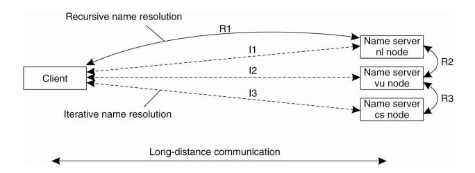
• Comparison between recursive and iterative name resolution with respect to communication costs.
