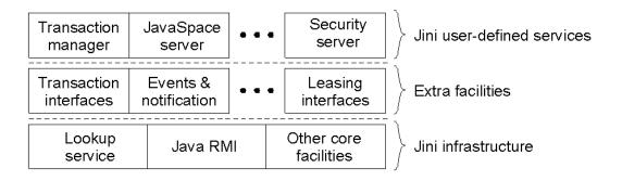
• The layered architecture of a Jini System.
