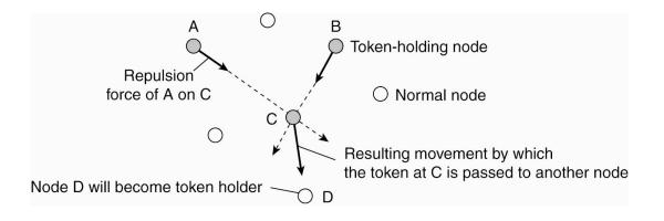
• Moving tokens in a two-dimensional space using repulsion forces.
