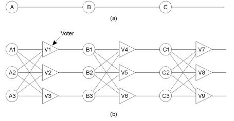
• Triple modular redundancy.
