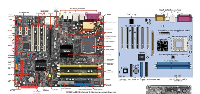
Picture of a motherboard/logicboard
