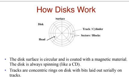
• Each track is split into *sectors* or *blocks*, the minimum unit of transfer from the disk.
