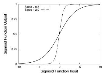
Fig. 1. Effects of steepness on two sigmoid functions:  $s_1 = 0.5$ ,  $s_2 = 2.0$ . Smaller s-values provide a greater ability to make subtle distinctions during training, but can lead to over-training.
