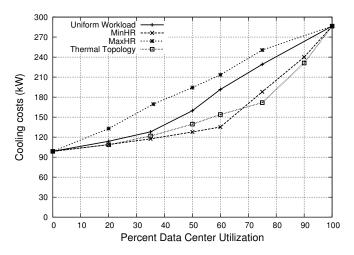
Fig. 6. Cooling costs for our three baseline algorithms and our thermaltopology-based algorithm. The Weatherman-based workload placement algorithm achieves savings comparable to the previous best in temperature-aware workload placement.
