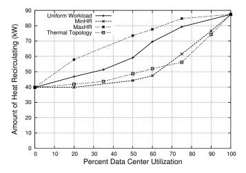
Fig. 5. Heat recirculation for our three baseline algorithms and our thermaltopology-based algorithm. Weatherman reduces the recirculation of hot air as well as, if not better than, the MINHR algorithm.
