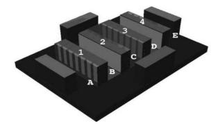
Fig. 2. Data center layout, containing 1120 servers in four rows of seven racks. The racks are arranged in a standard hot-aisle/cold-aisle configuration [4]. Four CRAC units push cold air into a plenum, which then enters the room through floor vents in aisles B and D. Servers eject hot air into aisles A, C, and E.
