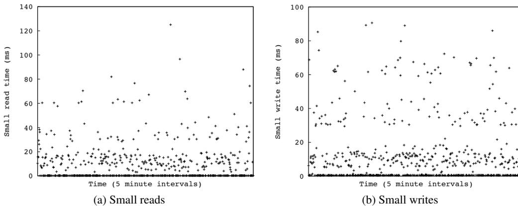
Figure 4: Jitter for small disk reads and writes.
