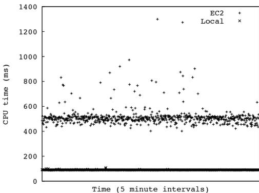
Figure 2: CPU jitter on an EC2 server.
