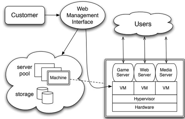
Figure 1: Cloud platform architecture.
