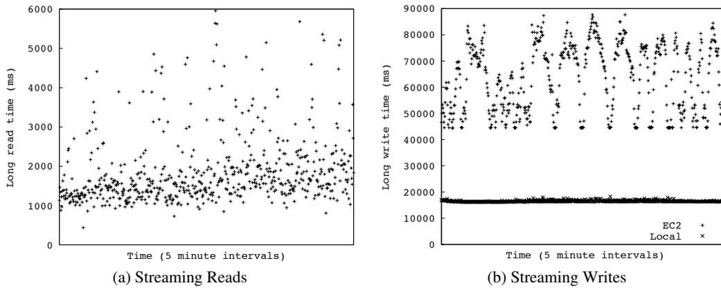
Figure 3: Jitter in disk throughput for large/streaming reads and writes.
