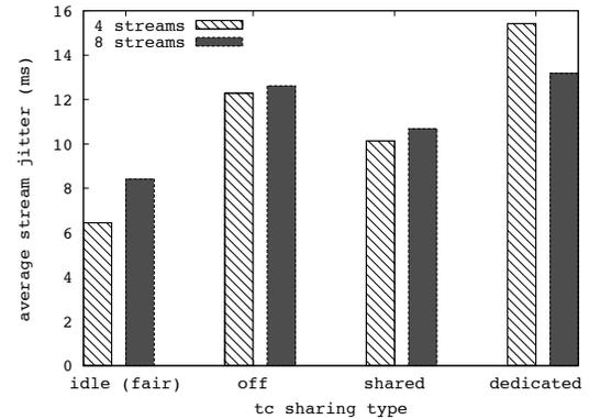
Figure 12: Stream jitter over 4 or 8 concurrent streams with a variety of network sharing setups.
