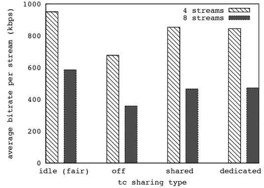
Figure 11: Average bit rate over 4 or 8 concurrent streams with a variety of network sharing setups.
