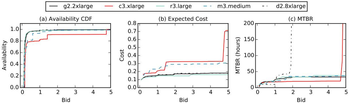
Fig. 2. The effect of bidding on availability, expected cost, and MTBR for selected instance types. Bids and the expected costs are normalized to a factor of the corresponding on-demand price.
